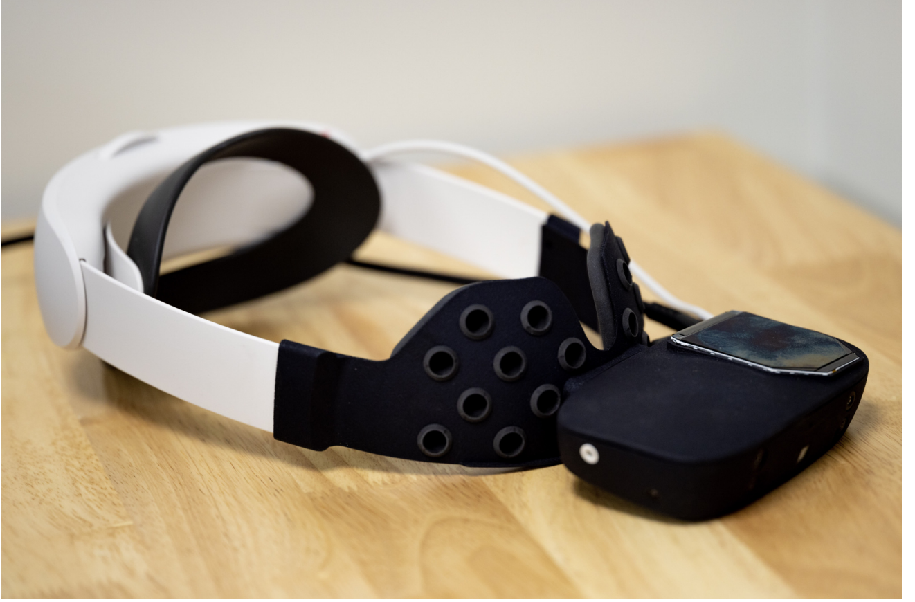
Fig. 2. The modified screen-free Quest 3 headset used to play ScOTT.
